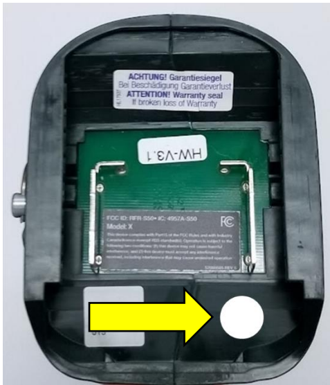
Figure 2 – Inspect Battery Shoe area to determine if White Dot Present (Arrow shows White Dot indicating Tool not affected)
