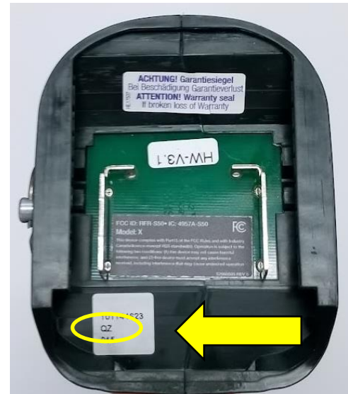
Figure 3 – Determine two-character Tool Date Code (Circle shows “QZ” in this example)
