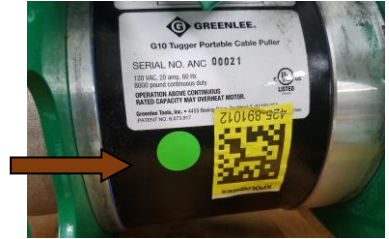
Figure 3 - Serial Number Plate w/ Green Dot Showing Software Update Completed
