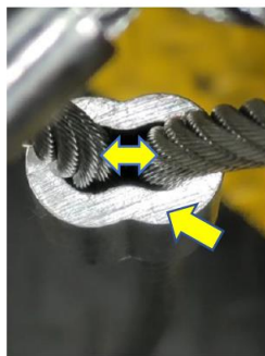
Fig 3. Sleeve Without Crimp Example Do Not Use
